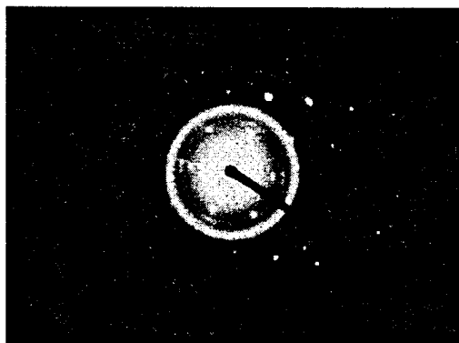
Figure 3. A TEM diffraction pattern shows polycrystalline diamond coating on the single crystal Si tip. A diffraction fringe of the polycrystalline SiC interfacial layer can also be seen inside the diamond ring.
