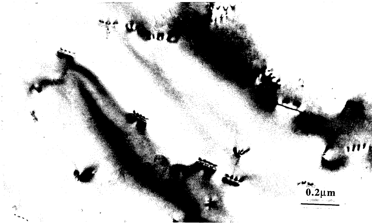
Figure 7. Low magnification plan-view bright field micrograph from the near surface region of the GaN film.
