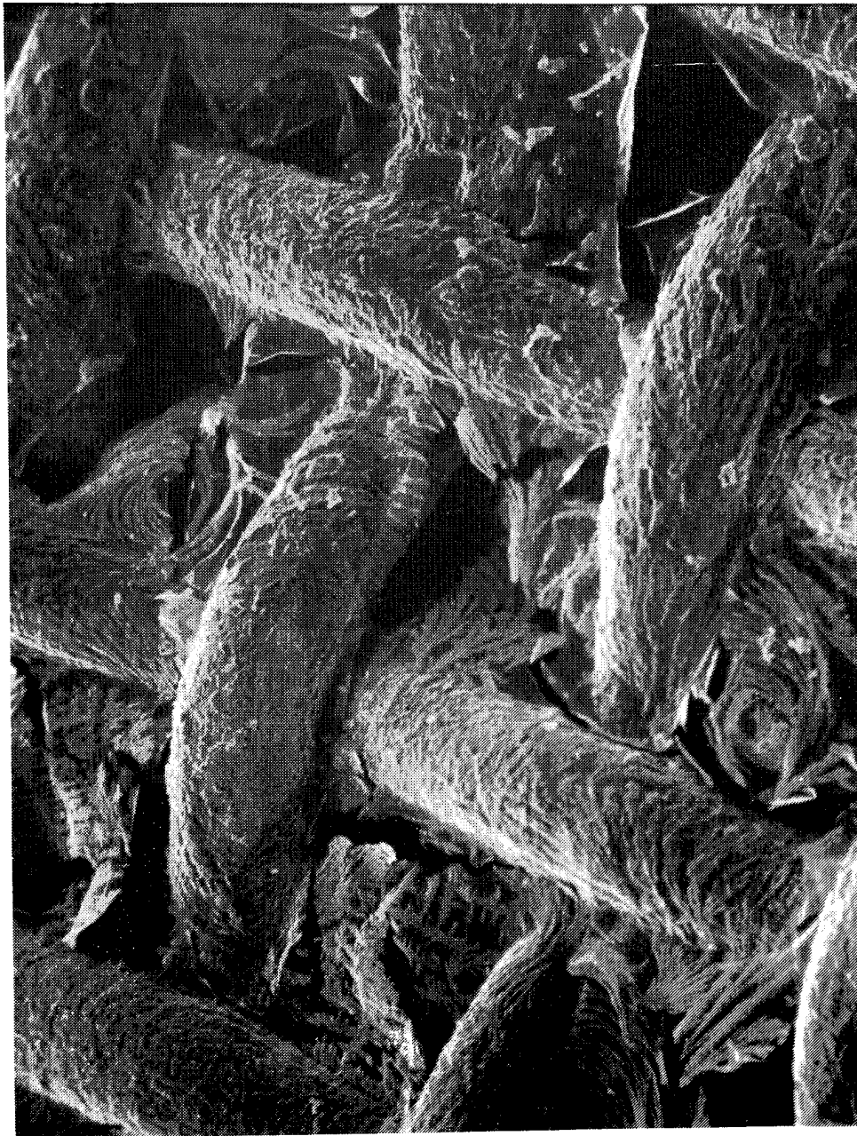
Figure 4-7. SEM of precipitate on a metal screen agitated in a poly p-phenylene terephthalamide/ H_2SO_4 solution. Magnification \approx 60X .
