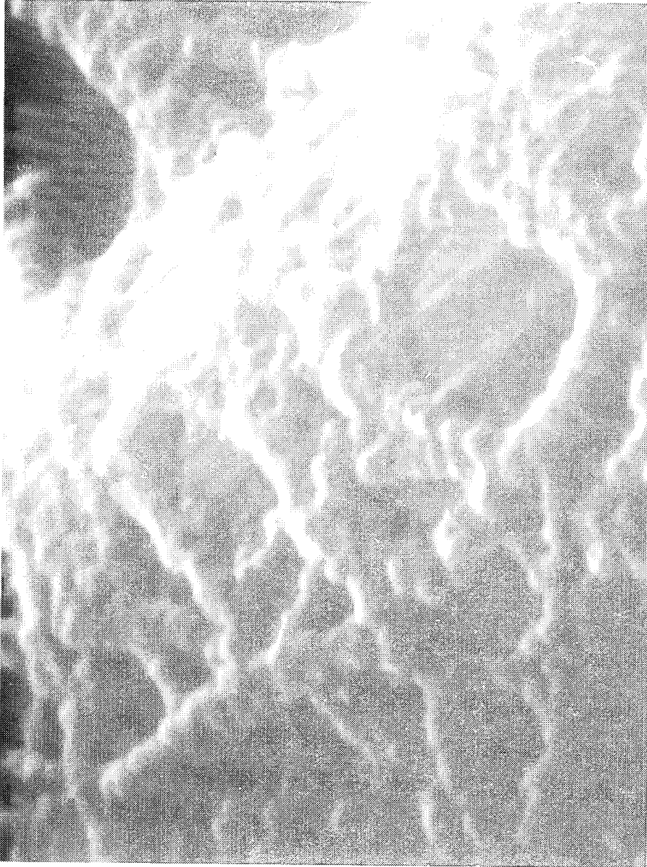
Figure 5-16. SEM of polypropylene In Situ Fibers deposited on graphite cloth from a 1.5 percent solution at 380 K (225°F). Magnification \approx 30,000X.
