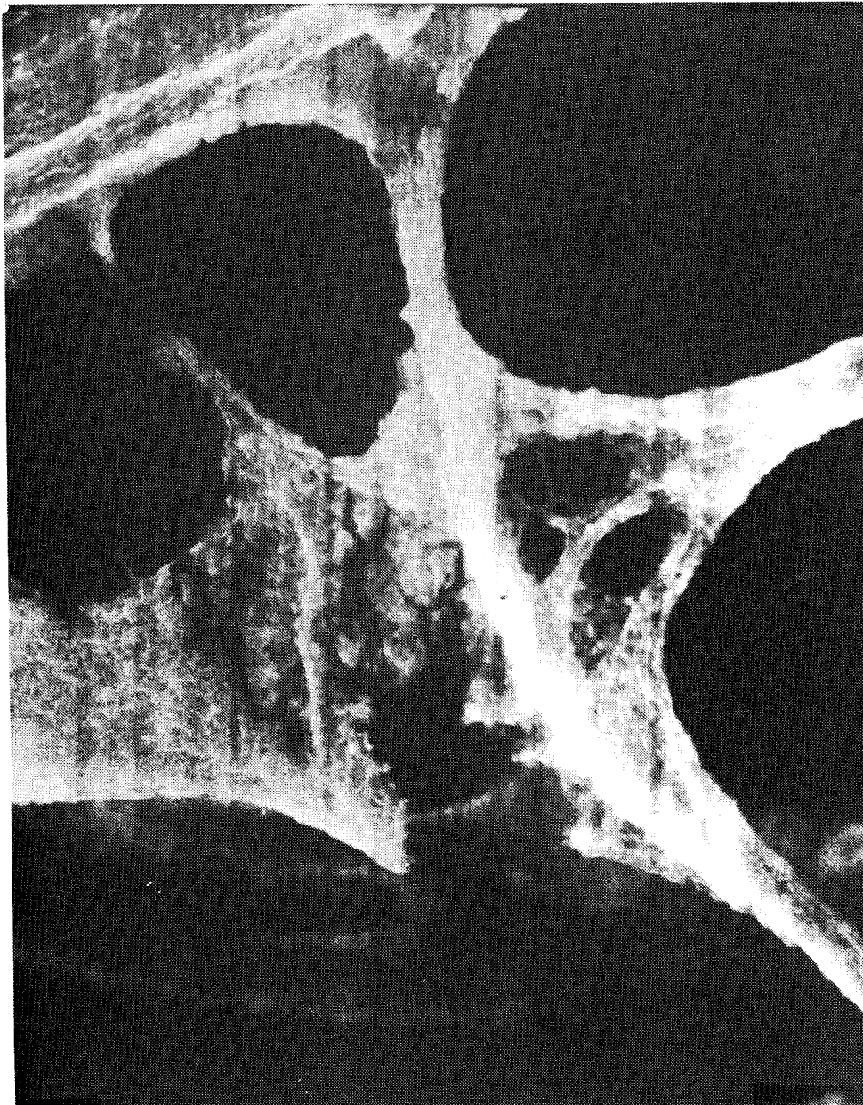
Figure 4-5. SEM of PCTFE fibers produced by In Situ Fiberization. Magnification \approx 1200X.
