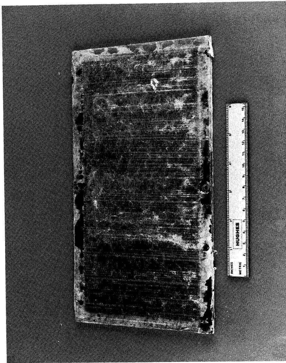
Figure 5-17. Typical fiberized array, 90° oriented graphite fibers.
