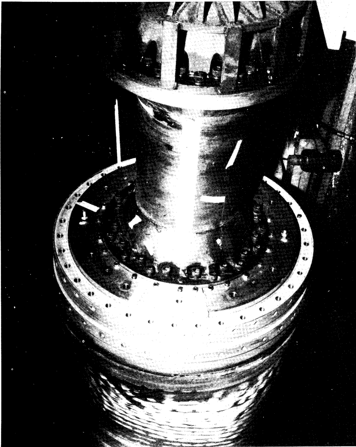
FIGURE 82. FINISH BONDED OUTER ADAPTER SLEEVE
