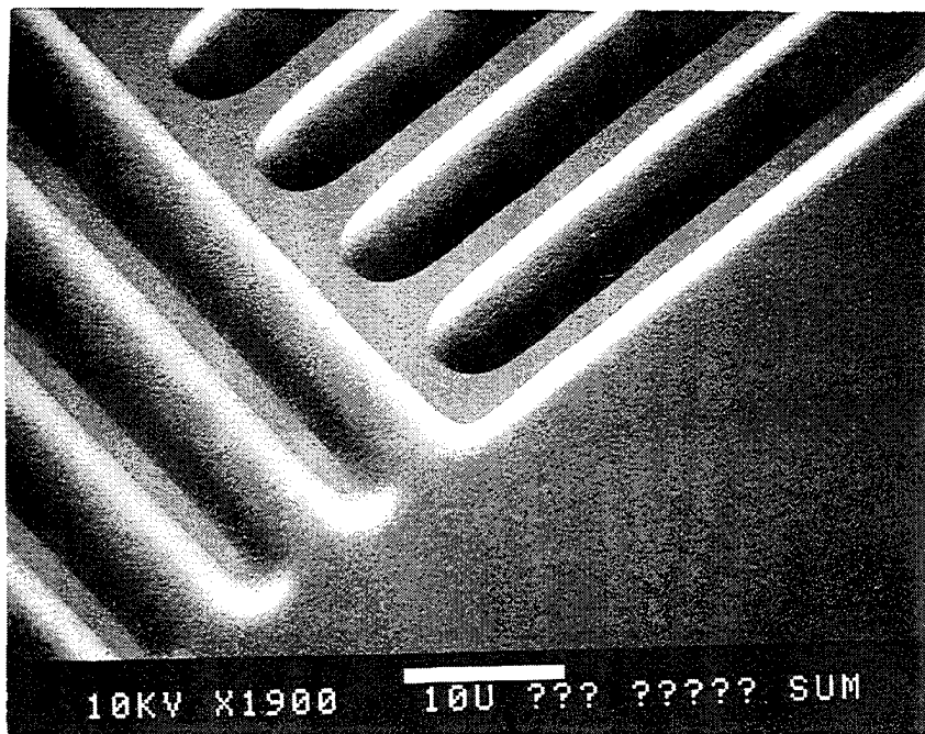
Fig. 6. Scanning electron micrograph of an exposure in 1.1 \mu\text{m} thick JSR IX 300 photoresist showing very good resolution of 4 \mu\text{m} lines and spaces.
