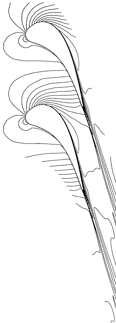
Figure 4: Mach contours at mid-span, i = 0^\circ incidence angle
