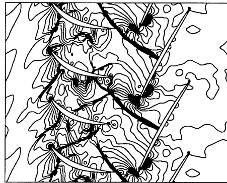
Fig. 14 - Instantaneous iso-pressure contours, Re = 400000 , configuration (A). Turbulence model used: Baldwin Lomax.
