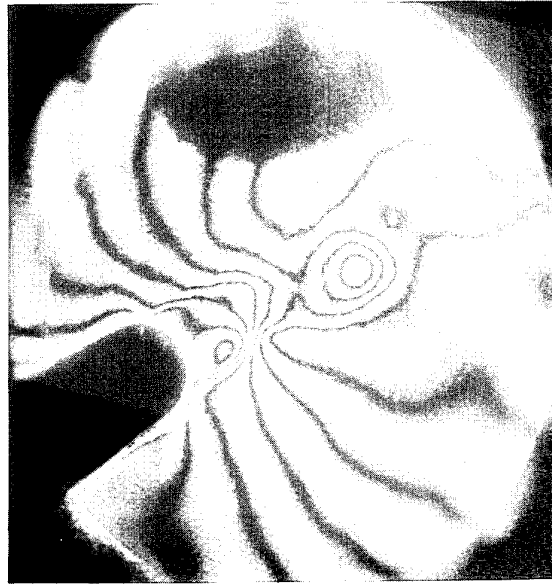
Fig. 6: Interferogram of the von Karman vortex street behind a large scale turbine guide vane at outlet Mach number M_2=0.4
