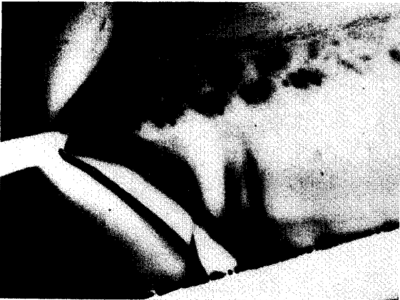
Fig. 2-c: Doublet: vortex shed 180° out of phase but as doublets (from Carscallen and Gostelow) [8]
