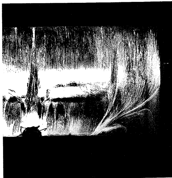
Figure 11: Wall streamlines on blade suction surface \lambda = 50^\circ, \alpha = 10^\circ
