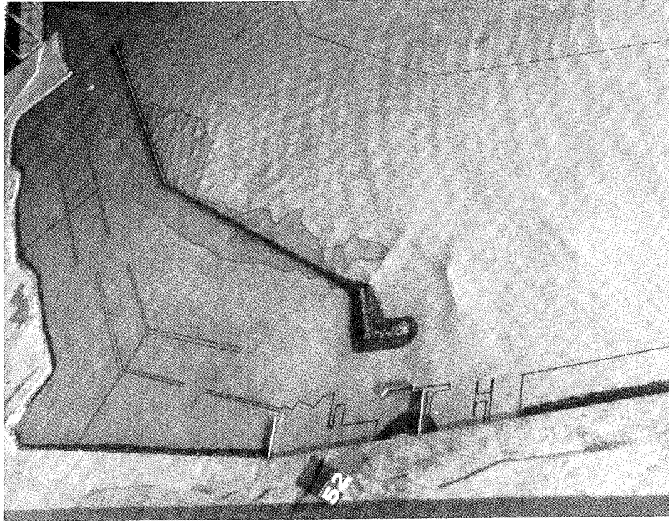
Photo 39. Typical wave patterns for Plan 6B; 12.5-sec, 8-ft test waves; swl = +8.0 ft
