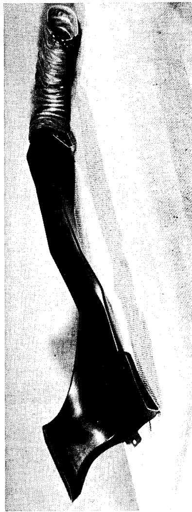
FIGURE 2: Heater duct for Ford Thunderbird, molded by Wiremold Company
