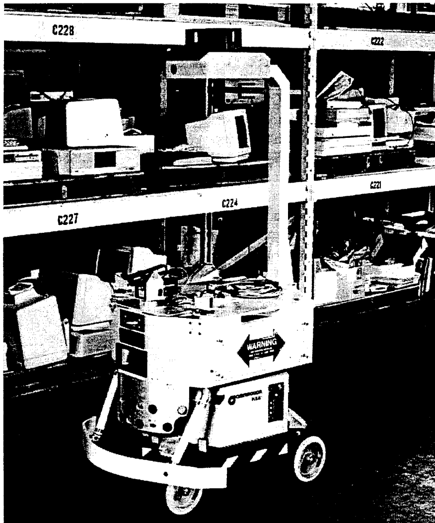
Figure 2. The prototype Cybermotion SPI module shown on the upgraded MDARS Interior robot patrolling in the Camp Elliott warehouse in San Diego.
