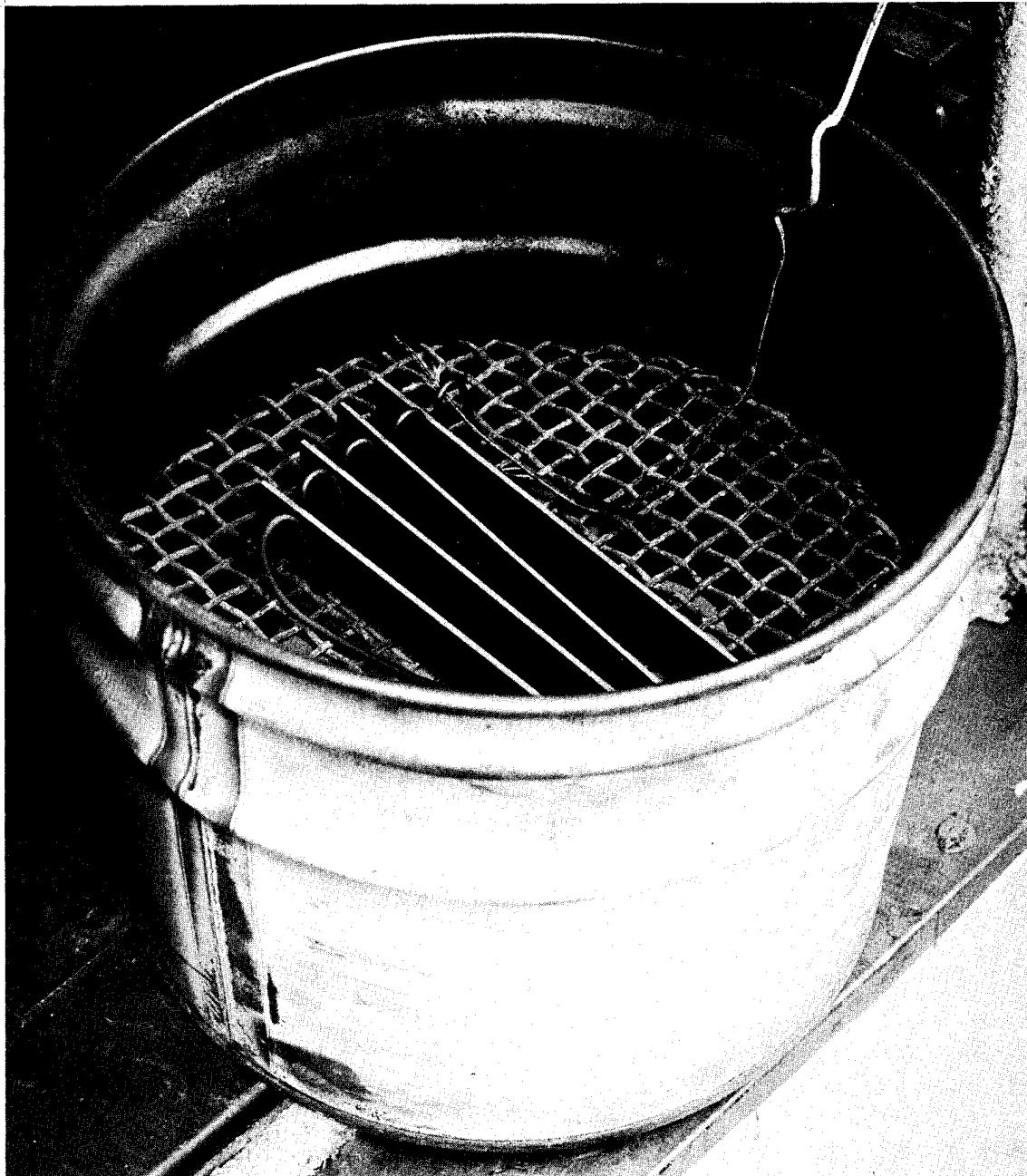
Figure 14. ITGA Specimens in Chamber Prior to Closing and Installation in Oven.
