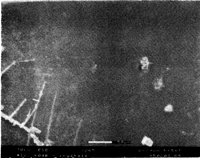
Figure 4. ESEM micrograph of 4340 steel with a PEG-060 coating exposed to the CG-59 bacterial consortia.
