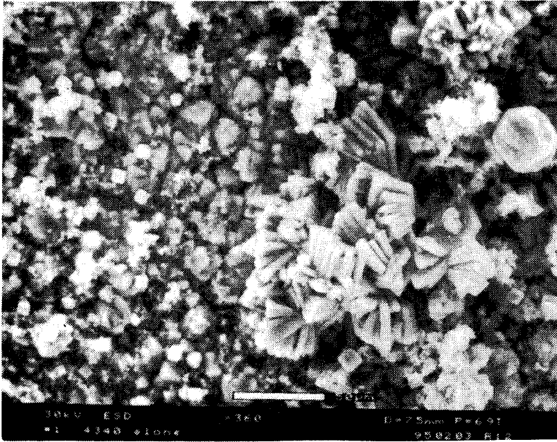
Figure 3. ESEM micrograph of untreated 4340 steel exposed to the CG-59 bacterial consortia.
