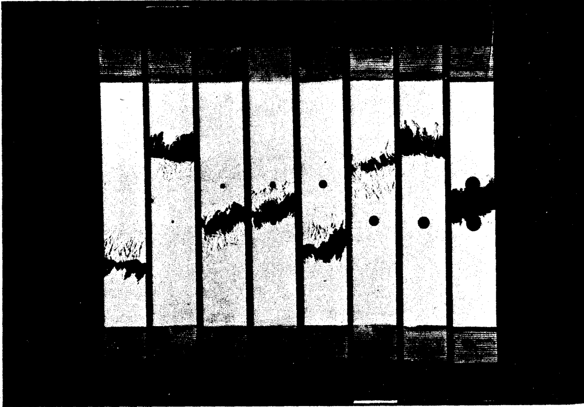
FIGURE 20. SMC-25 FRACTURED NOTCH SENSITIVITY SPECIMENS
