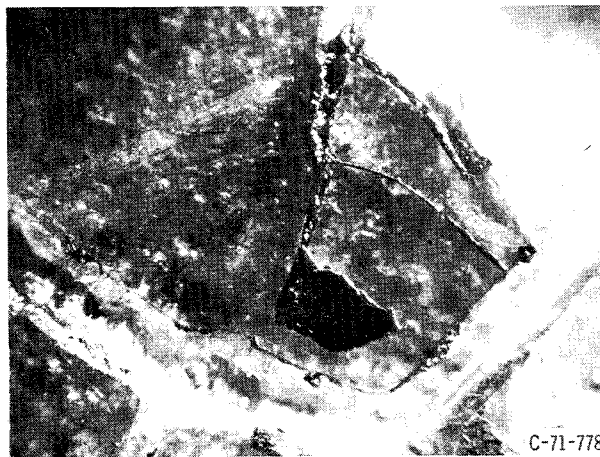
(c) Severe thermal degradation.
