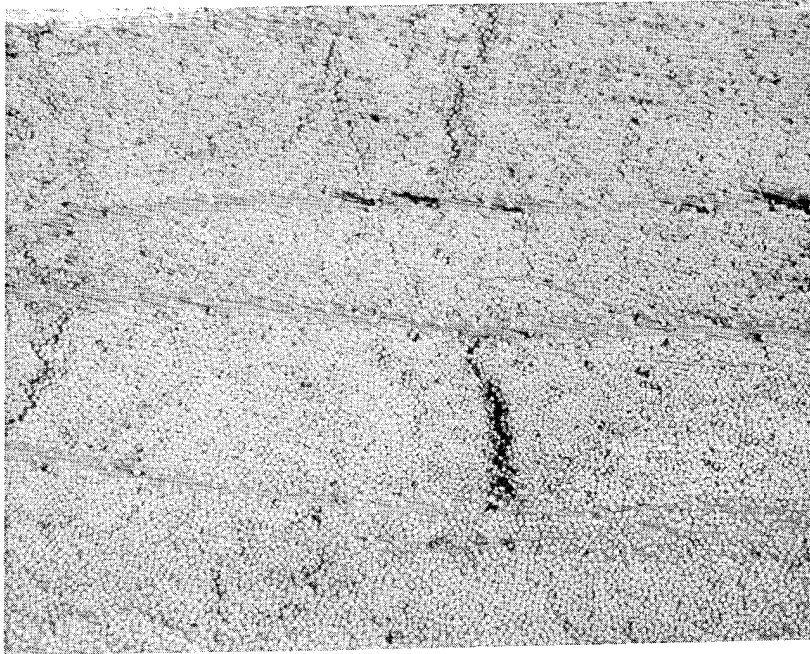
FIGURE 3. Cross Section Photoenlargement of Laminate C, Table 7 (X100)
