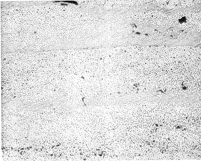
FIGURE 6. Cross Section Photoenlargement of Laminate F, Table 7 (X100)
