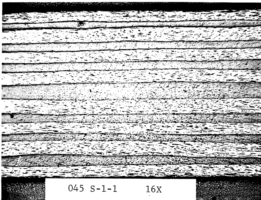
Fig. 13 PHOTOMICROGRAPH OF LONGITUDINAL SECTION OF 0 \pm 45^\circ PR-286/ MODMOR II GRAPHITE/S-GLASS (1:1) COMPOSITE CONTILEVER BEAM SPECIMEN AFTER BEING SUBJECTED TO 5 \times 10^5 SHEAR FATIGUE STRESS CYCLES (MAX. \pm 2 KSI, R = -1)
