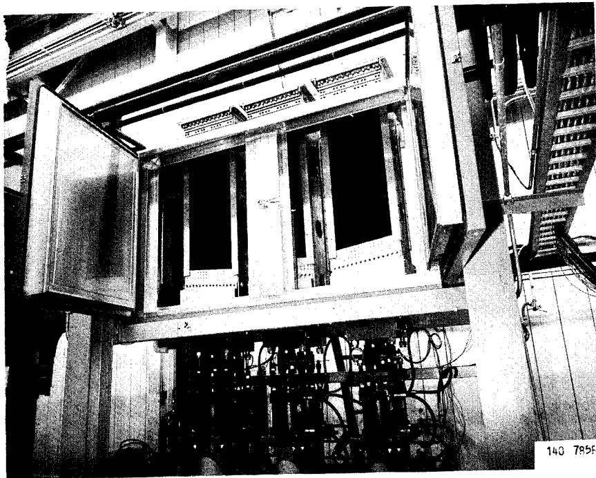
Figure 16. - Six covers in an environmental chamber.
