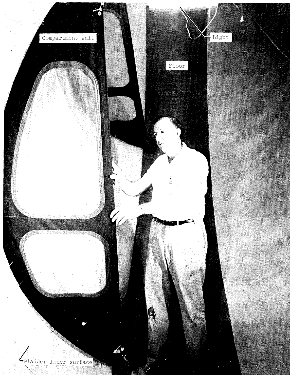
Figure 3.- Internal view of 24-foot-diameter torus.
