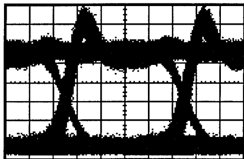
Fig. 3 The eye diagram of the transmitter at 130°C.
