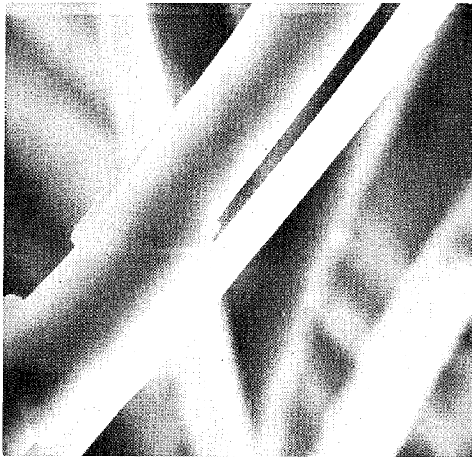
FIGURE 31. 2210X SEM - PRD-49 FILAMENT SHOWING MODE OF FAILURE ON TENSILE SIDE OF IMPACT SURFACE PANEL #5, MODULITE 5206/PRD-49
