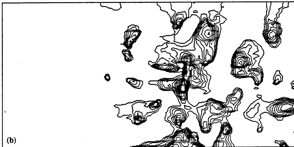
Figure 9: Wall contours at t = 0.50 msec: (a), low streamwise momentum; (b), high pressure.
