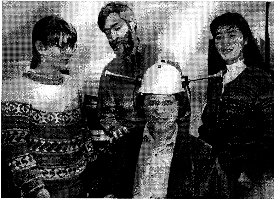
Fig. 1. The M.I.T. pseudophone configured to present supernormal interaural delays.
