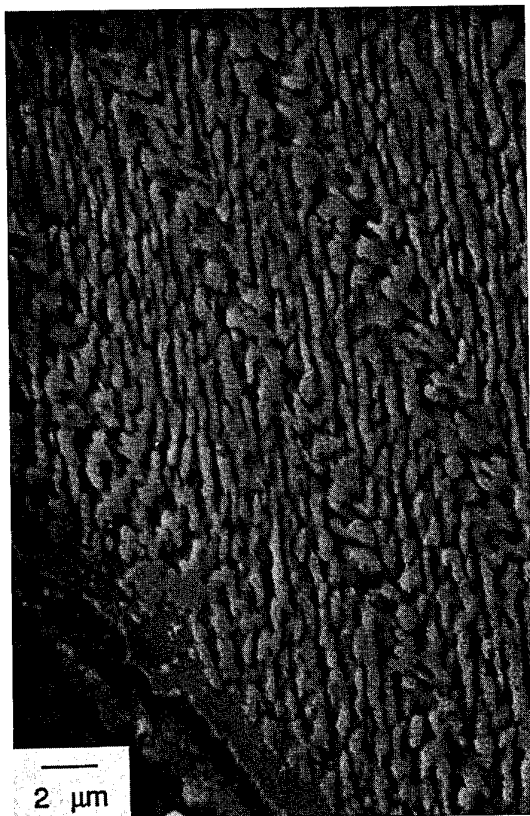
Fig. 5: \gamma' -morphology after TMF-loading, out-of-phase, 400-1000°C, \Delta\epsilon_m = 1.04\% , Raftening parallel to stress axis and slip bands adjacent to crack. SEM. Oxalic acid etching.
