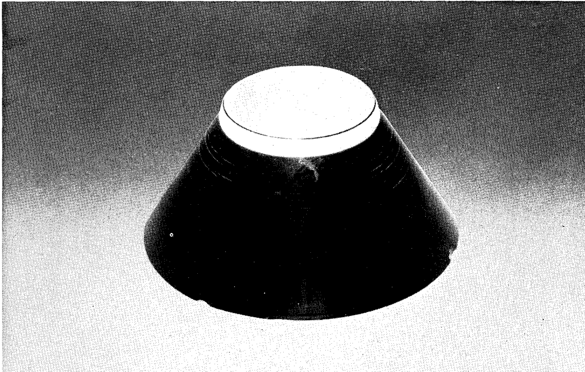
Figure B-8. Arrested failure of 1-inch-diameter, 60^\circ , 1.0 t/D ratio window at 22,000 psi, low-pressure face. (Phase 1 of deformation.)
