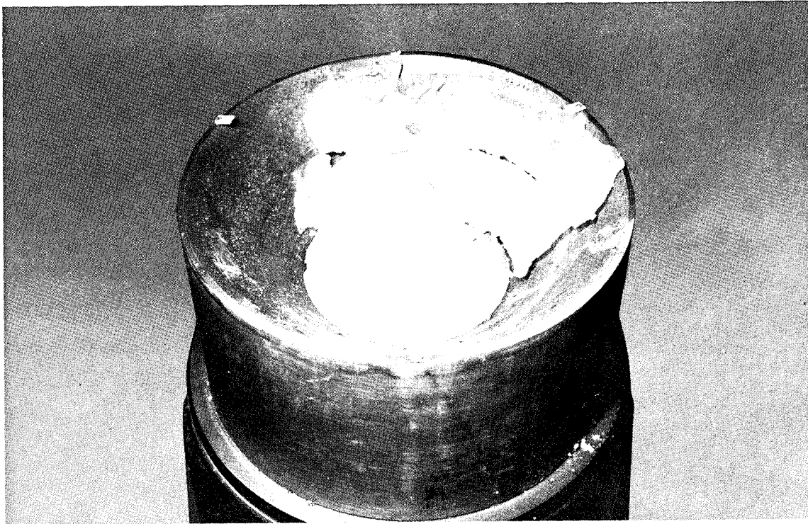
Figure B-45. Failed 8-inch-diameter, 90°, 0.5 t/D ratio window, high-pressure face, shown in mounting flange.
