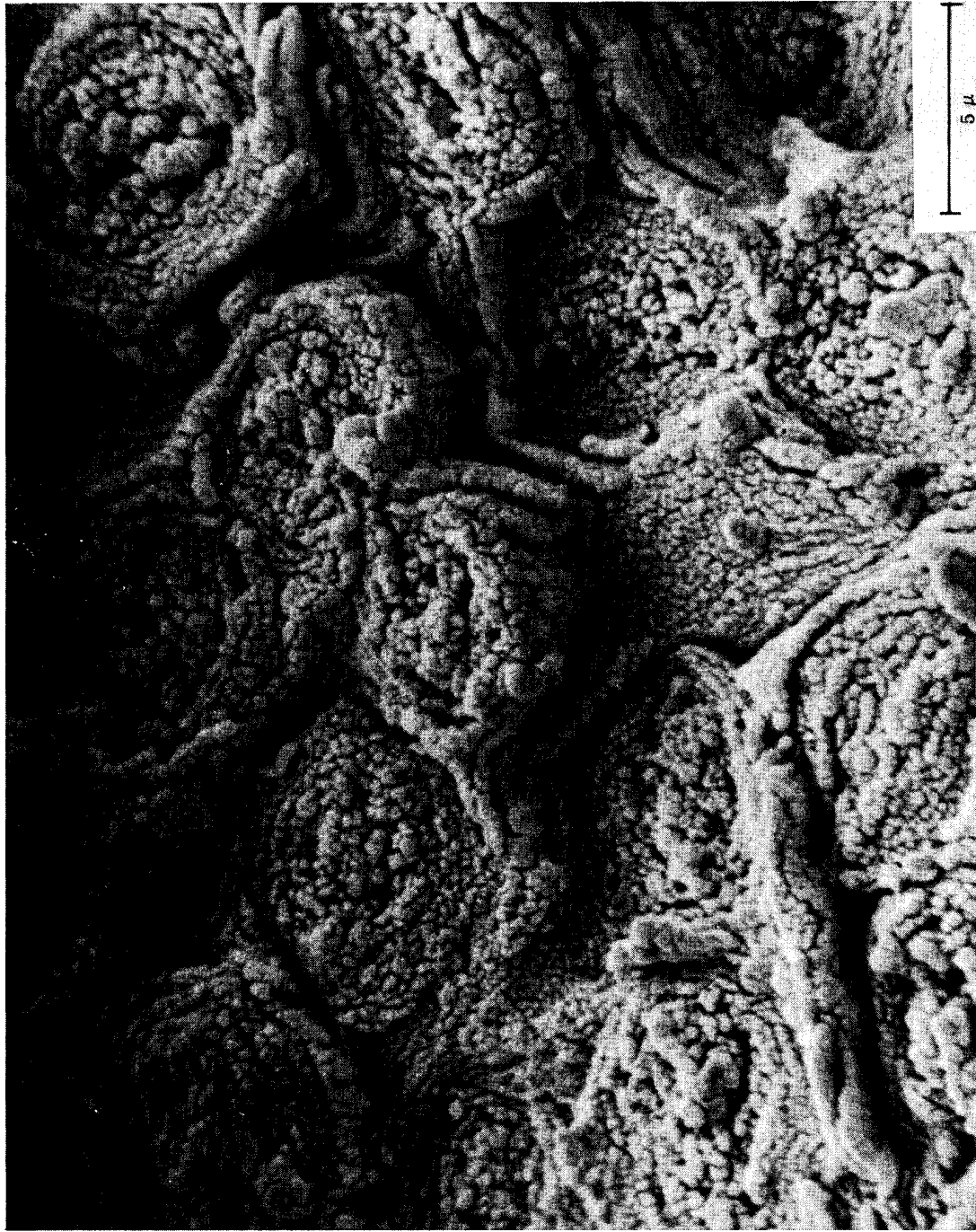
Figure 12. - Fracture Surface of 1273°K Type-C Tow in GW-173, Copolyrised to 1673°K, Heat-Treated to 2873°K, 6100X, Fiber Tensile Strength = 0.615 GN/m 2 (89,000 psi)
