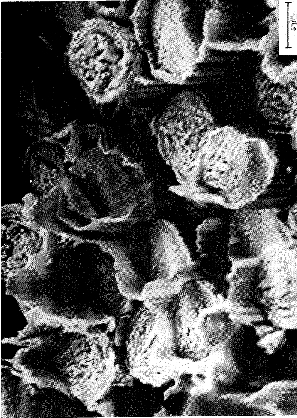
Figure 13. - Fracture Surface of 1273°K Type-C Tow in 396 Pitch, Copolylysed to 1673°K, Heat-Treated to 2873°K, 5000x, Tensile Strength = 0.97 GN/m 2 (140,000 psi)
