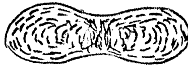
Figure 38. - Schematic Microstructure of Fully Graphitized Type-D Tow. The microstructure illustrates the typical wrap-around basal orientation of fully stabilized and graphitized fibers
