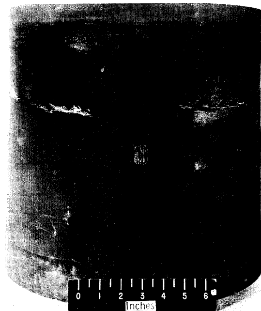
Figure 7.- Cylinder failed in compression at elevated temperature. Cylinder 42.
