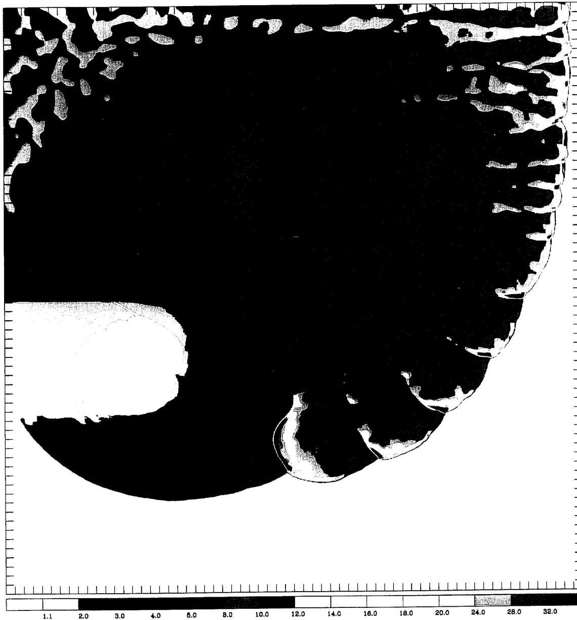
Figure 5(a): Simulated pressure contours showing reignition of detonation at an area expansion. The area map filling and contouring scheme was used to indicate the various pressure levels.
