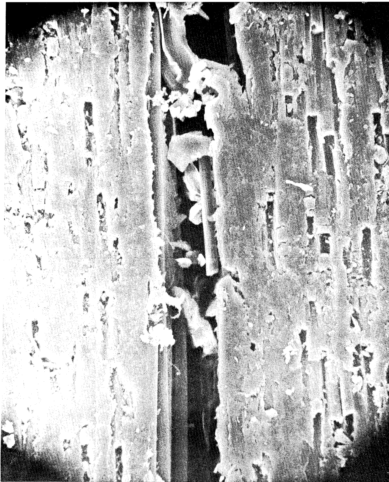
Figure A-15: ELECTRON PHOTOMICROGRAPHS OF ILS TEST FAILURE AREA, LAMINATE 17, TABLE 8. X300
