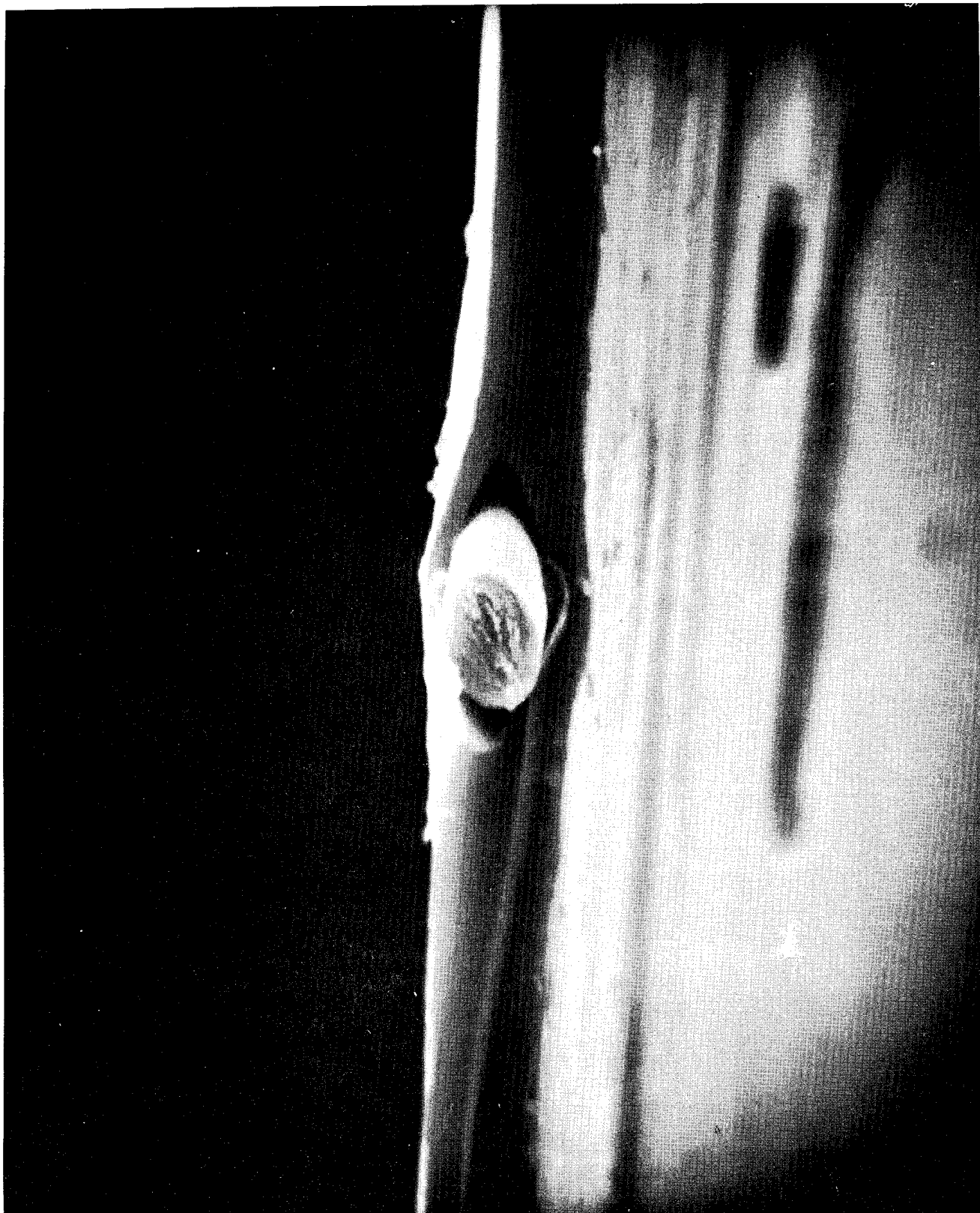
Figure A-5: SCANNING ELECTRON PHOTOMICROGRAPHS OF "SINGLE" GRAPHITE FIBERS IMPREGNATED IN 1:3 BLOCK COPOLYMER (POLYMER 12, TABLE 2) X1400
