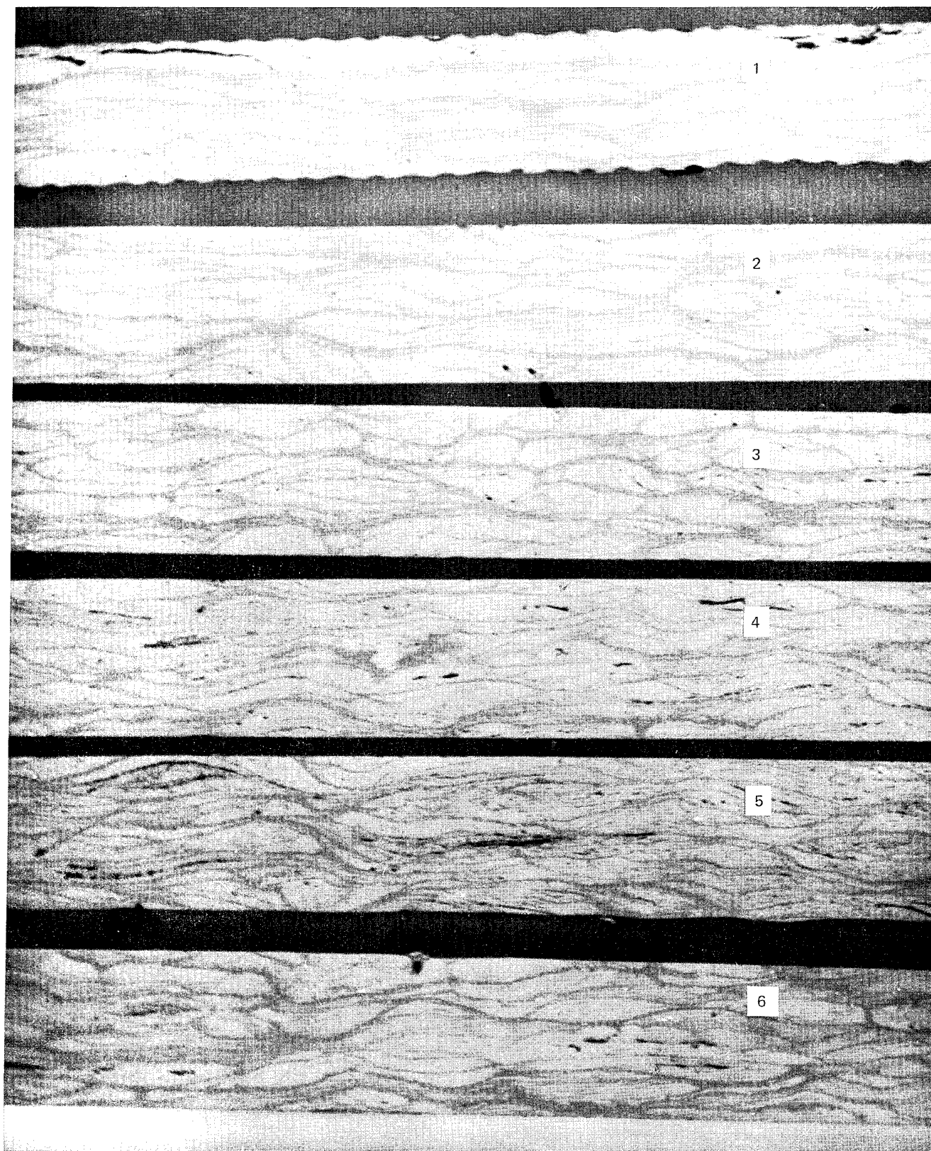
Figure 9: CROSS SECTION PHOTO ENLARGEMENTS OF LAMINATES 1 THROUGH 6 (TABLE 8). X 10
