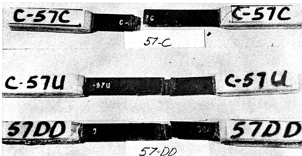
FIGURE II.24. UNIAXIAL COMPRESSION SPECIMENS 57-C, U, DD AFTER FAILURE, [0/90_2/0]_3T
