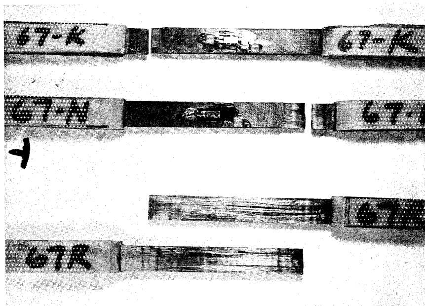
FIGURE II.16. TENSILE SPECIMENS 67-K, N, R AFTER FAILURE, [0/90_2/0]_{3T}
