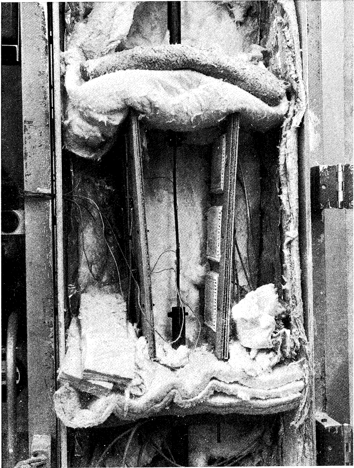
FIGURE 22.—CREEP AND RUPTURE TEST SETUP
