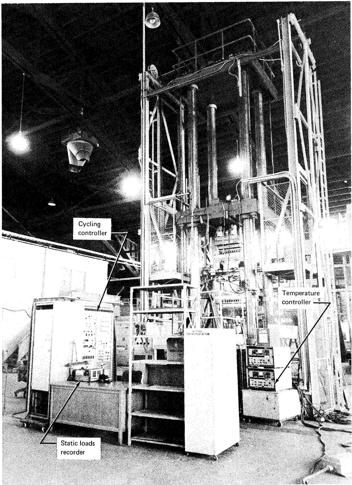
FIGURE 32.— 150-KIP ELECTROMECHANICAL RESEARCH FATIGUE MACHINE
