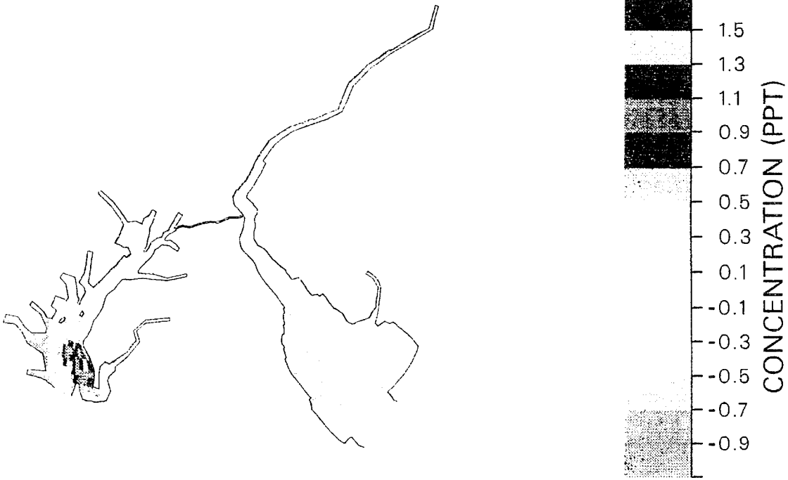
Figure 30b. Differences of seasonal averaged salinity (highest-low, 1977) due to proposed channel deepening in layer 16 (0.8 m)
