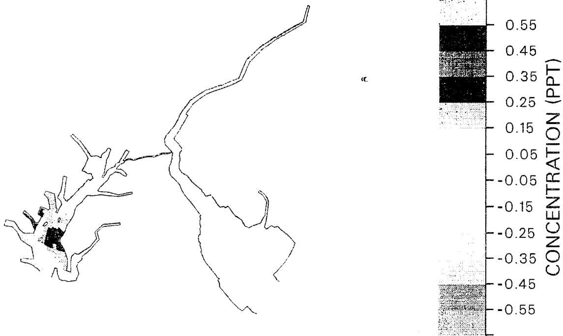
Figure 33d. Differences of seasonal averaged salinity (lowest-low, 1964) due to channel deepening test 2 in layer 16 (0.8 m)
