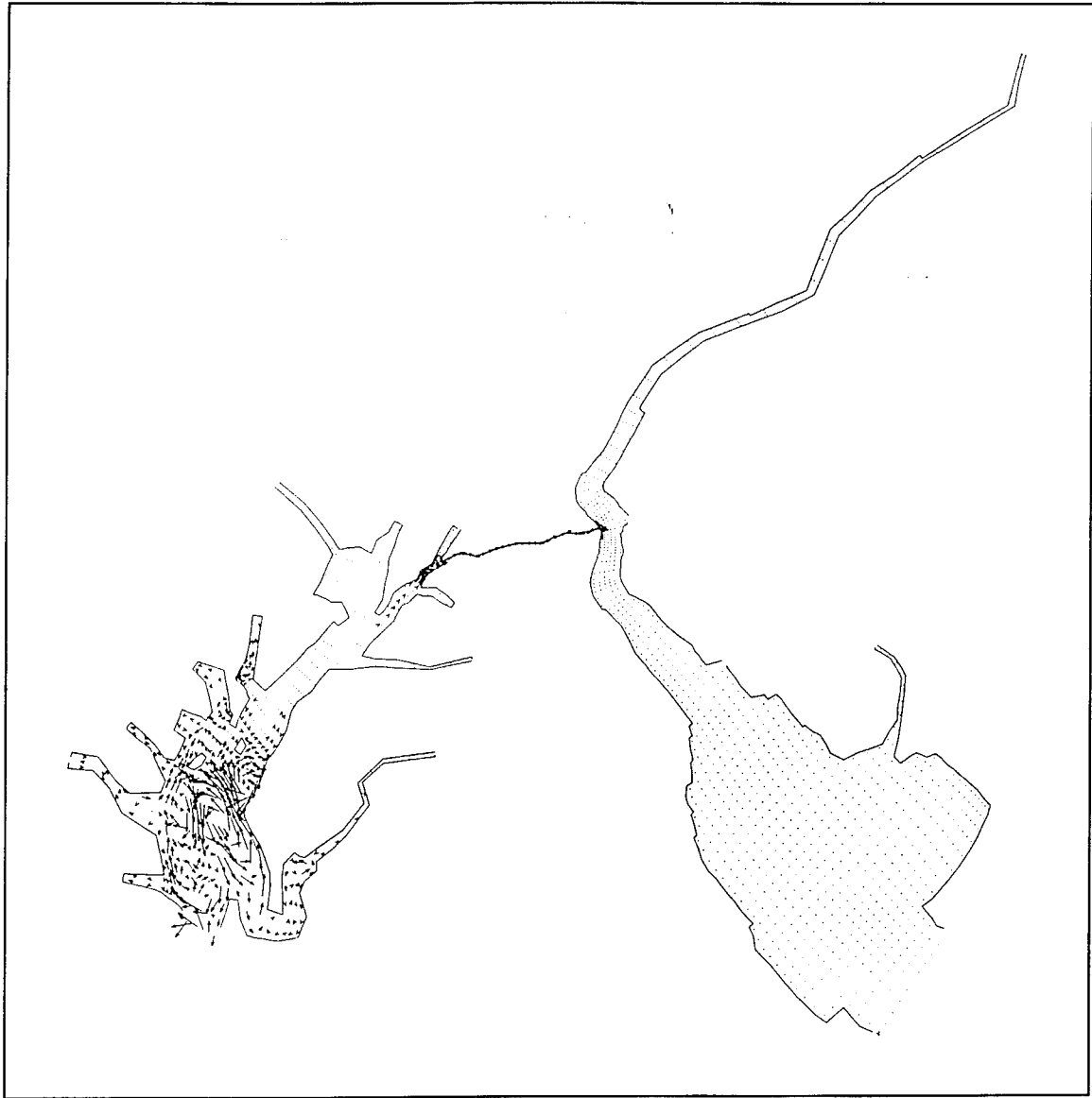
Figure 34c. Differences of seasonal averaged flow (highest-low, 1977) due to channel deepening test 2 in layer 16 (0.8 m)
