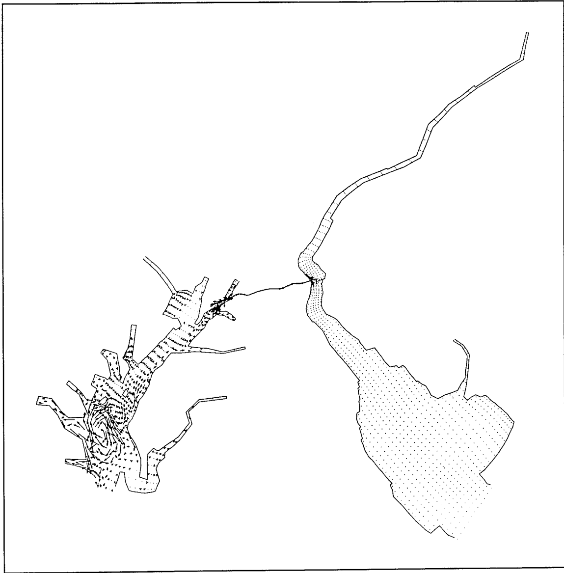
Figure 29a. Differences of seasonal averaged flow (lowest-low, 1964) due to proposed channel deepening in layer 16 (0.8 m)
