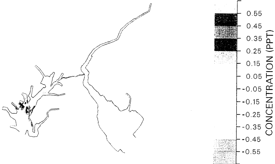
Figure 29b. Differences of seasonal averaged salinity (lowest-low, 1964) due to proposed channel deepening in layer 16 (0.8 m)
