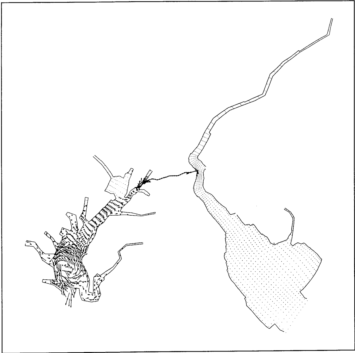
Figure 30a. Differences of seasonal averaged flow (highest-low, 1977) due to proposed channel deepening in layer 16 (0.8 m)
