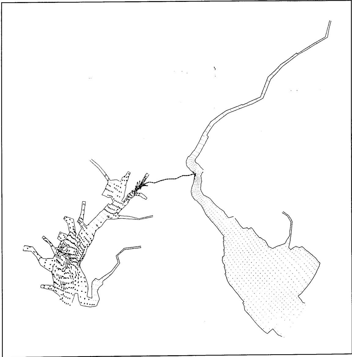
Figure 33a. Differences of seasonal averaged flow (lowest-low, 1964) due to channel deepening test 1 in layer 16 (0.8 m)
