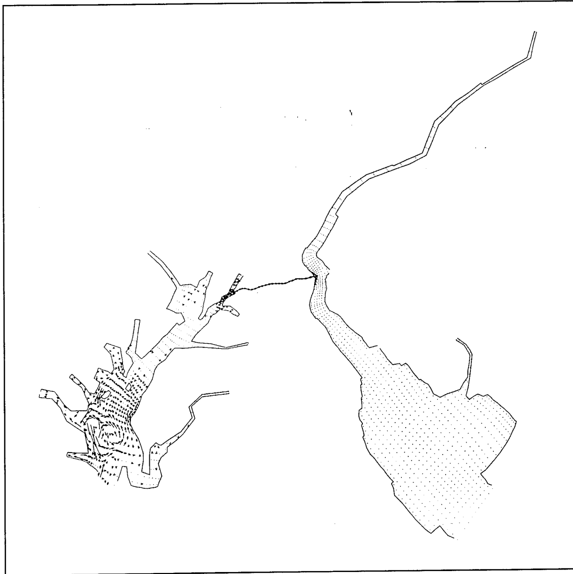
Figure 33c. Differences of seasonal averaged flow (lowest-low, 1964) due to channel deepening test 2 in layer 16 (0.8 m)
