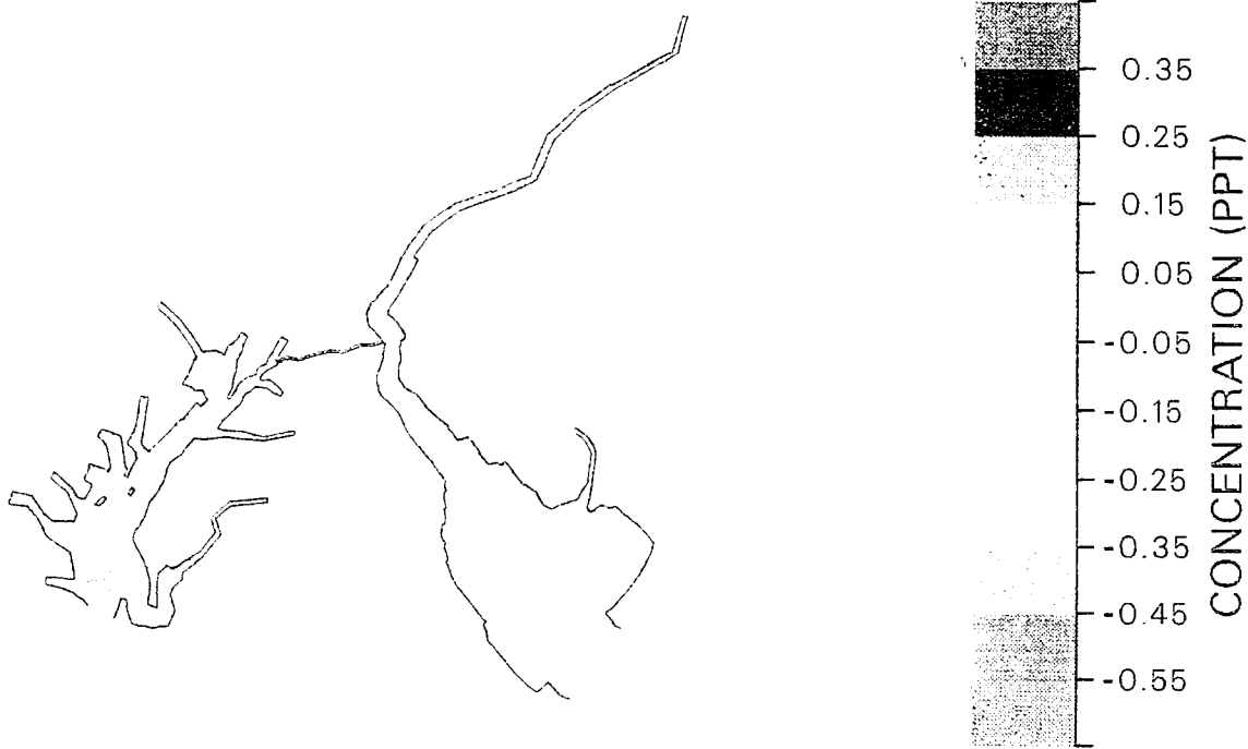
Figure 35b. Differences of seasonal averaged salinity (highest-high, 1972) due to channel deepening test 1 in layer 16 (0.8 m)
