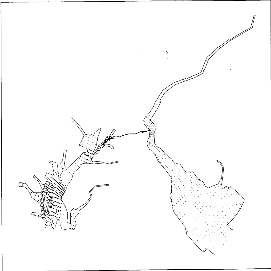
Figure 35a. Differences of seasonal averaged flow (highest-high, 1972) due to channel deepening test 1 in layer 16 (0.8 m)
