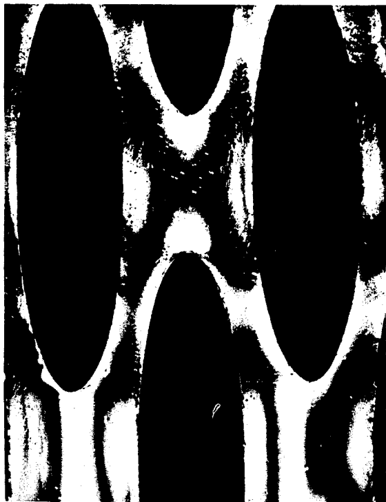
Figure 58. Photoelastic Patterns for Elliptical Holes and Solid Inclusions (50% Volume Fraction) with Load Applied Along Major Axis Direction
