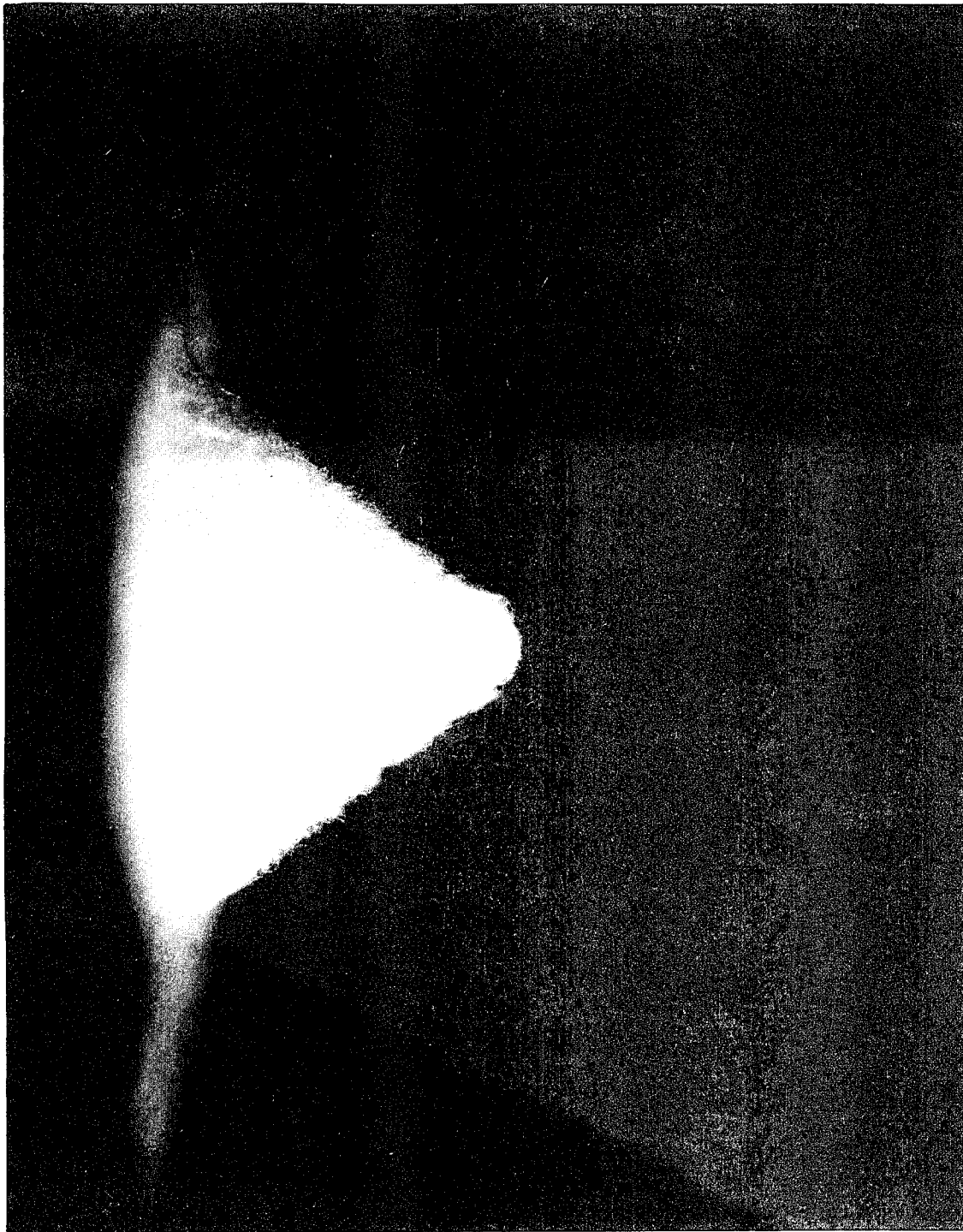
Figure 2. Response of Non-Woven Nylon Felt during Ballistic Impact. 230 Microseconds after Impact by 17-Grain Fragment Simulator. Initial Velocity - 650 feet per second. Felt - 43 ounces per square yard.
