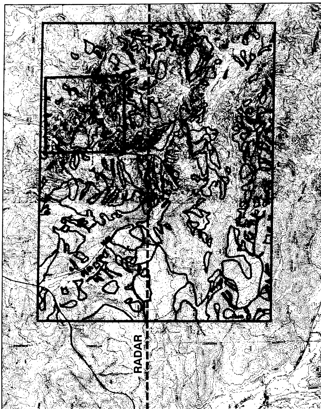
Figure 3.1-3: Landslide inventory map produced for the study area. The topographic base includes portions of the USGS 7.5-minute Clayton (1980) and Antioch South (1980) quadrangles
