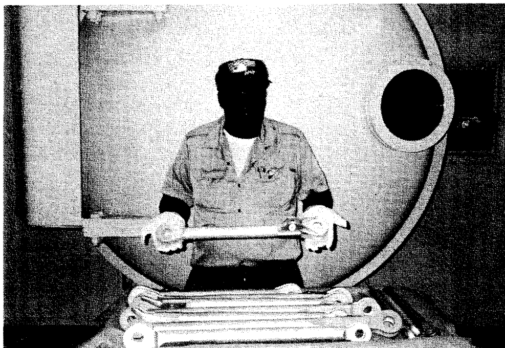
Figure 17. Typically Processed Warner Robins Steel Parts After IVD Aluminum and Glass-Bead Peening.
