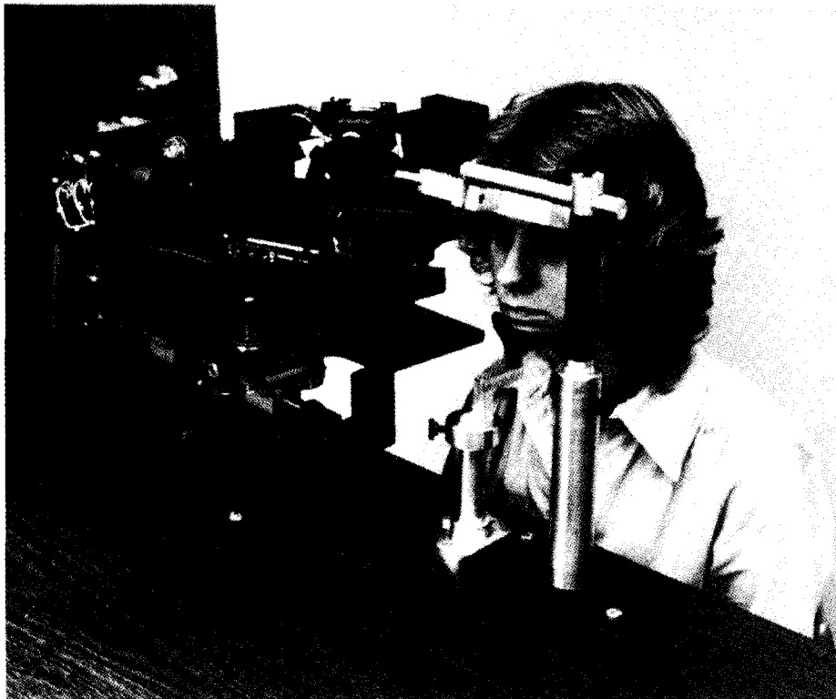
Figure 6.8 SRI International dual Purkinje image eye tracker, from Crane and Steele (ref. 17).
