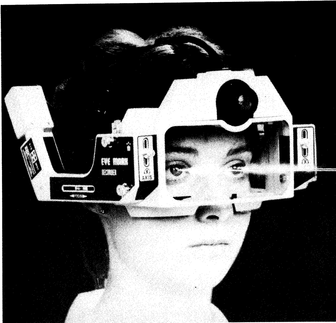
Figure 6.4 NAC corneal reflex tracking system, from reference 16.
