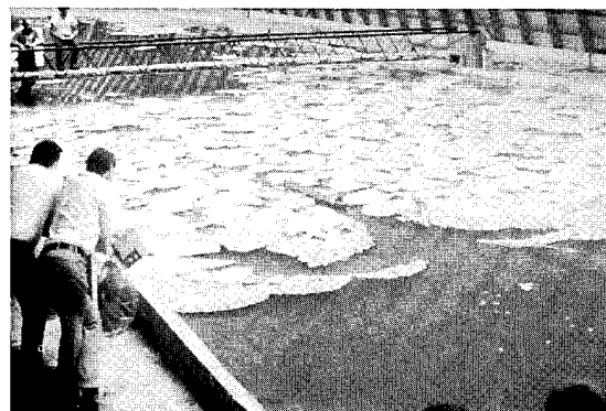
Figure 15. Physical model study using MOD-ICE.
