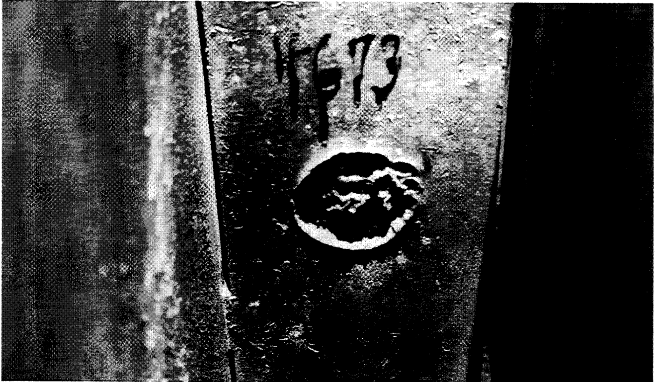
Figure 12. Photograph of crater on interior wall of RHA test fixture formed by impact from thin copper disk.
