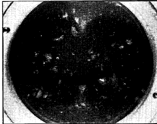
Front-Coated DAR-1 / REP / ms-ZnS: 10 min @ 210 m/s
