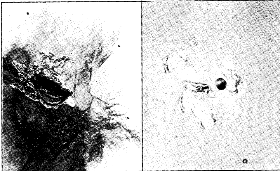
DAR/REP-2 (10 min @ 210 m/s) Nomarski micrograph (93×) Surface/subsurface damage/delamination
