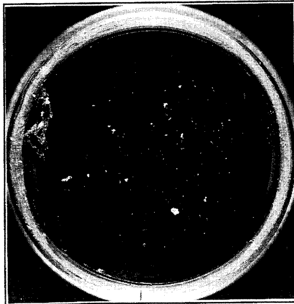
FIGURE 17. Whirling Arm Rain Exposure of Antireflection-Coated Bulk GaP (Sample I15-D) in Run 5 at 210 m/s in a 25.4 mm/h Rainfall of 2-mm-Diameter Drops at Perpendicular Incidence. This sample was exposed to 500°C for measuring optical properties prior to the rain erosion test.
