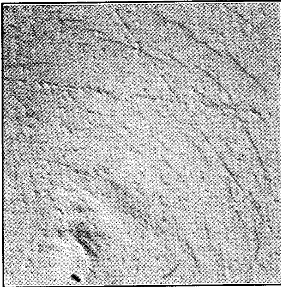
MgF 2 : 10 min @ 210 m/s Nomarski micrograph (360x) showing ring fracture
