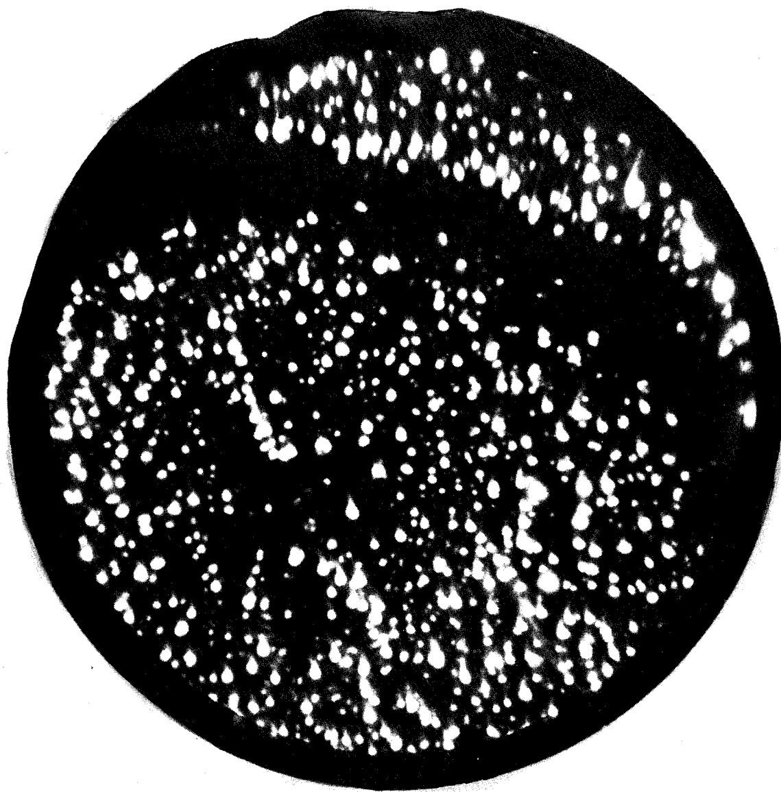
Figure 7. - Tungsten after PTFE contact (16.2 kV, helium image gas, liquid helium cooling).
