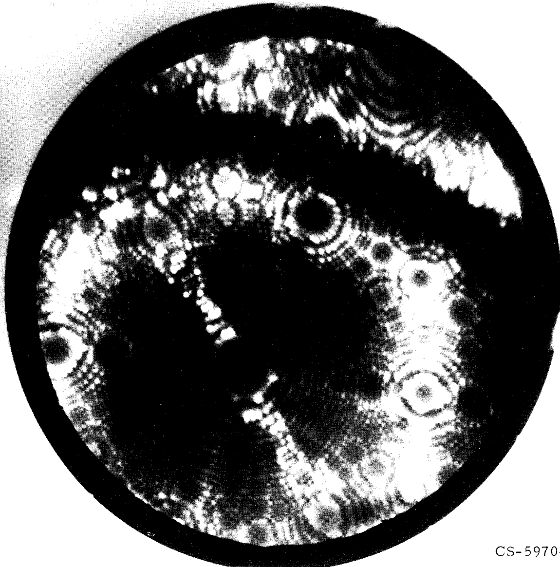
Figure 6. - Tungsten prior to contact (18.0 kV, helium image gas, liquid nitrogen cooling).
