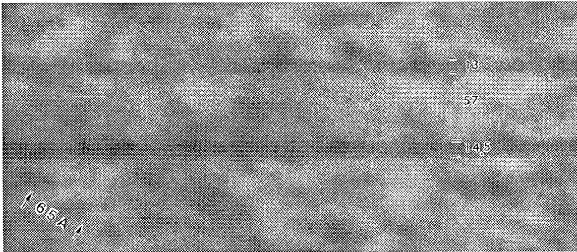
Fig. 4.3. High resolution TEM lattice image showing the layer morphology. The arrows show 20 (111) GaAs lattice spacings of 3.26 \text{ \AA} each. The total spacing between the arrows is 65 \text{ \AA} .
