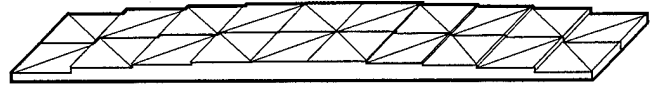
Figure 8.—Optimum shape of simply supported beam with constant thickness across width. Excitation frequency f_{ex} = 270 Hz.
