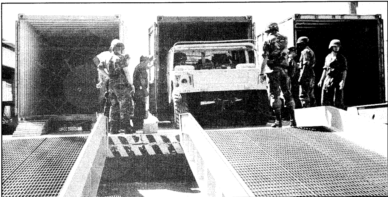
A High Mobility Multipurpose Wheeled Vehicle (HMMWV) Is Driven Into a 40-Foot Container at Fort Carson, Colorado, as Part of the Loading Portion of United States Transportation Command's Turbo Intermodal Surge 1995 Exercise. Two HMMWVs or a Combination of Vehicles and Trailers Were Loaded Into Each 40-Foot Container.
