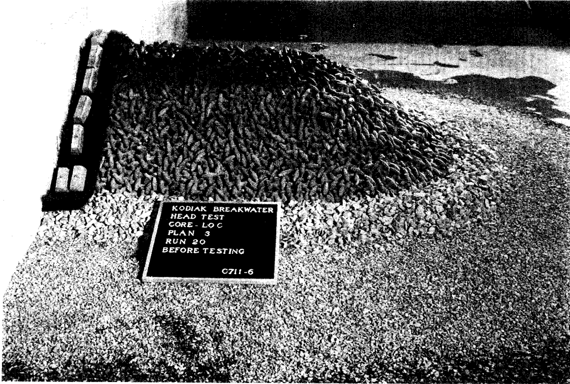
Photo 11. Sea-side view of model breakwater Plan 3 before testing
