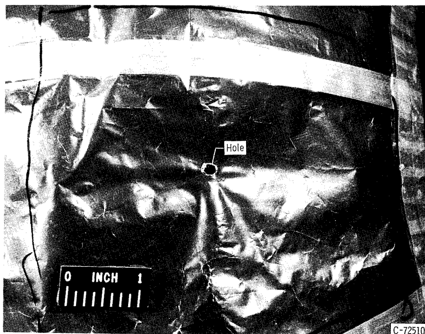
Figure 13. - Leak in liner 5 (Mylar laminate) in upper dome.
