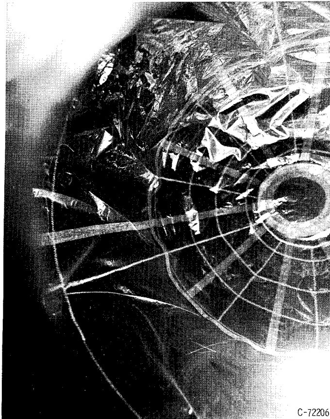
Figure 12. - Liner 5 (Mylar laminate) after failure. Photograph taken with liner in place.
