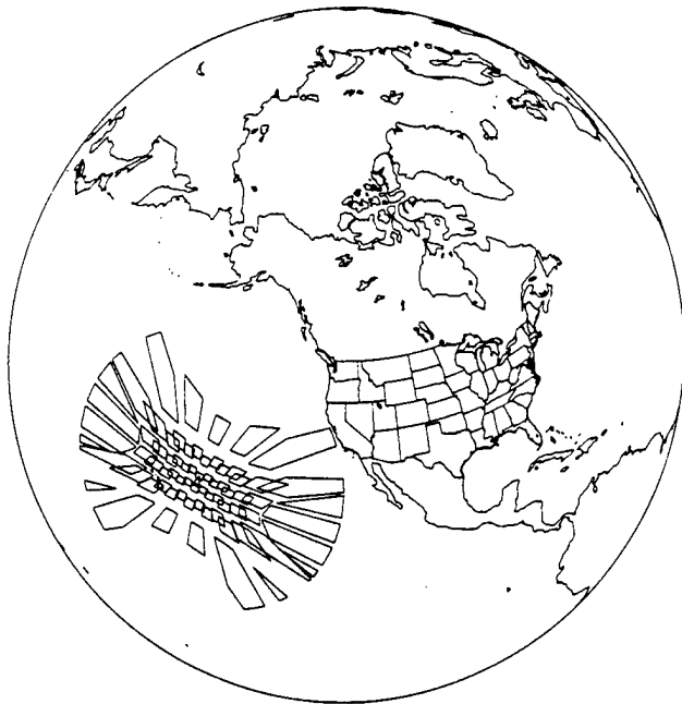
Fig. 6 The viewing geometry of MAXIE at several positions within one scan.
