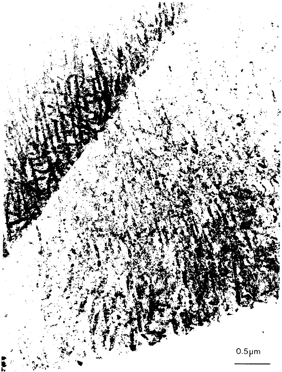
Figure 6 Low magnification bright field image showing densely populated hydride present in the equiaxed \gamma grains of duplex 48-2-2 charged at 13.8MPa.
