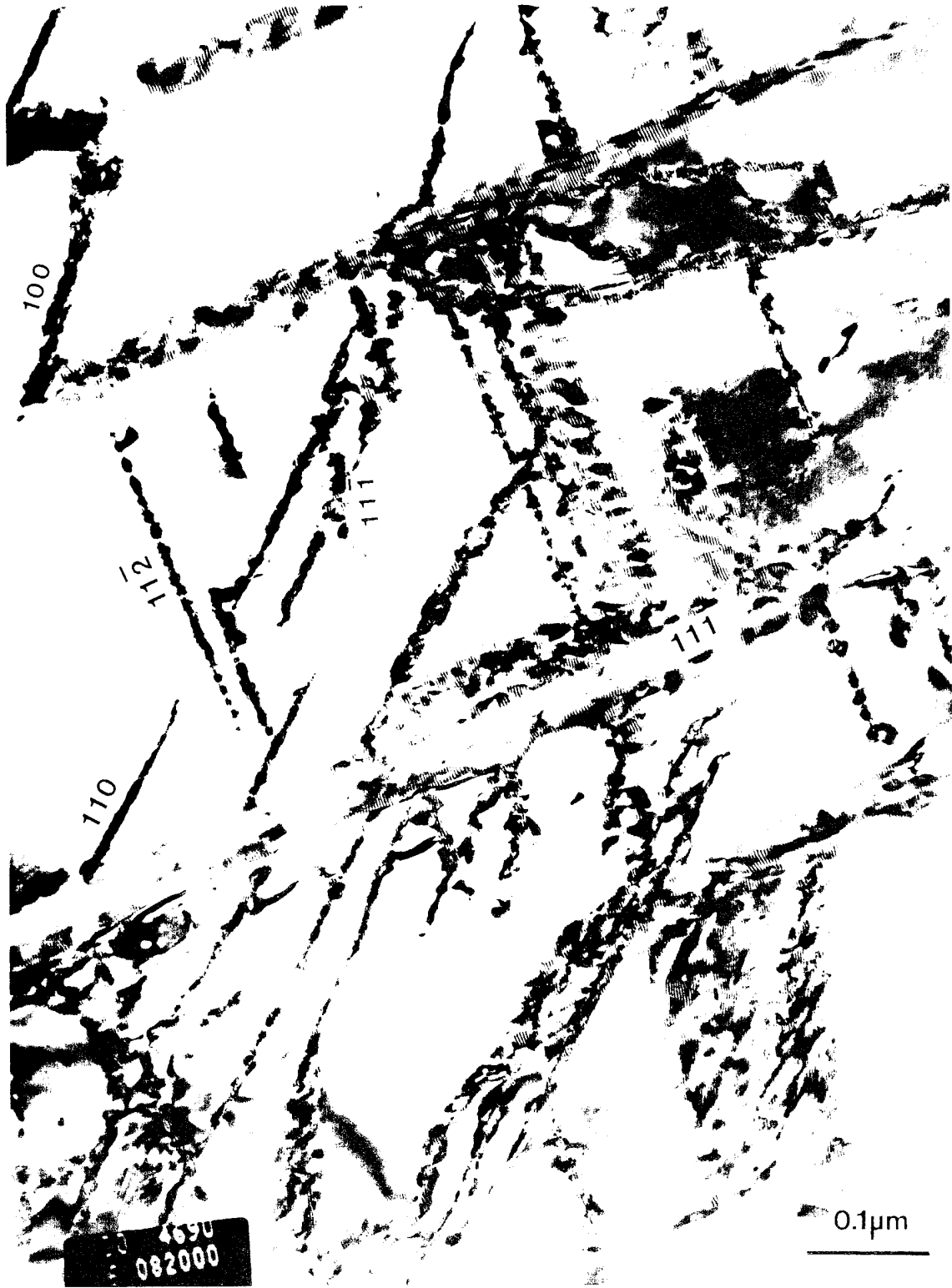
Fig. 32 TEM BF image of lamellar 48-2-2 charged at 13.8 MPa showing FCC hydrides.
