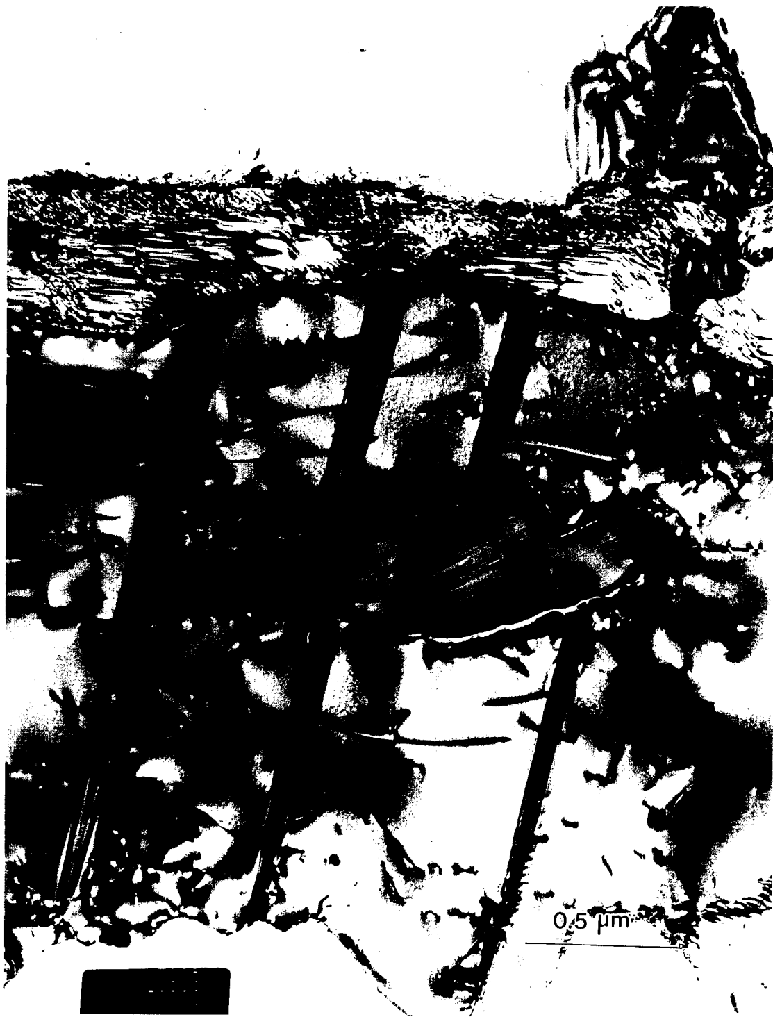
Figure 4 Isolated precipitate of the new hydride is embedded in the \gamma -grain with twins.
