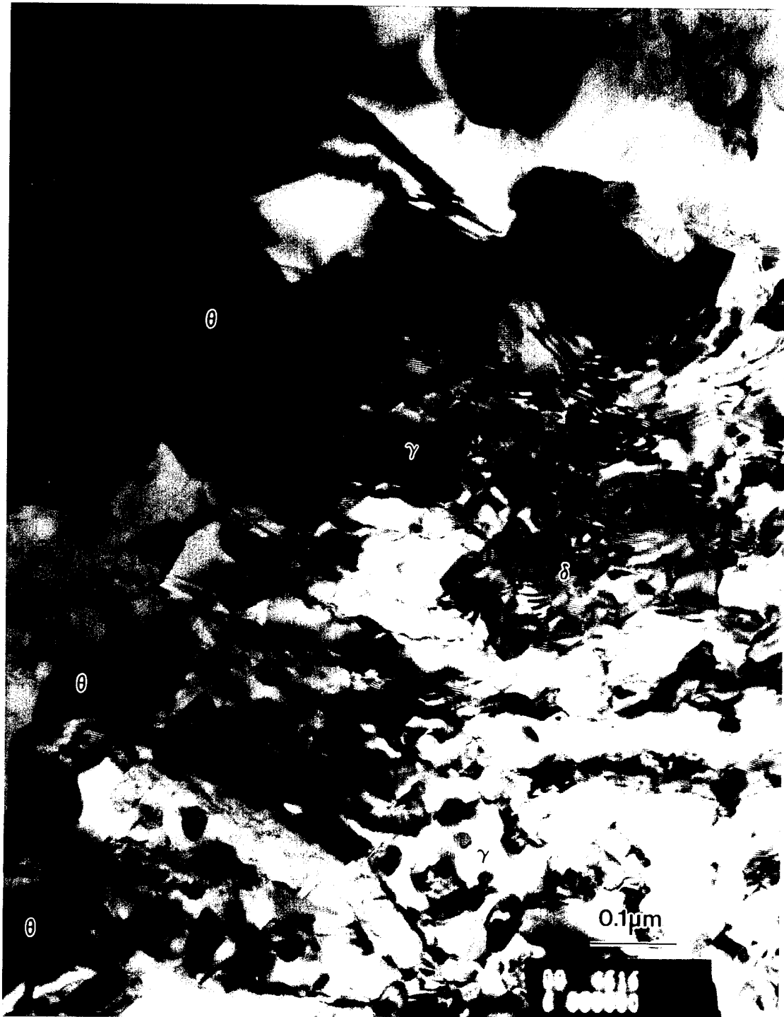
Figure 5 TEM bright field image showing densely populated FCC hydrides and few tetragonal hydride grains are present at duplex 48-2-2 following charging at 13.8MPa and 800°C.
