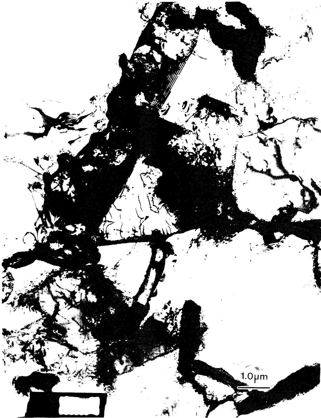
Figure 8 Hydride phases surrounded by dense dislocations are present along \gamma grain boundaries.
