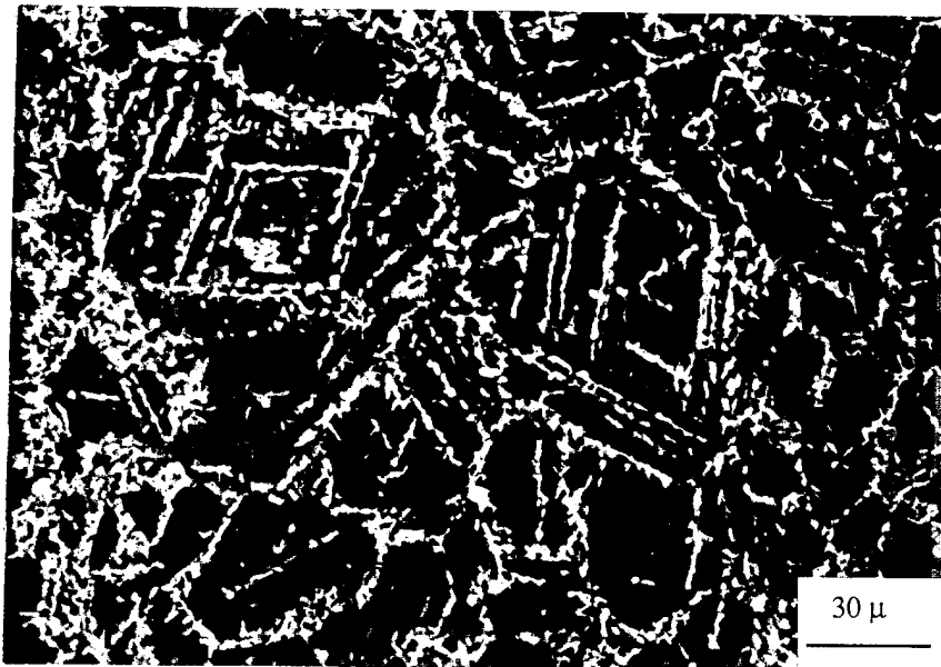
Figure 3 - Duplex microstructure following charging at 800°C and 13.8MPa for 60 hrs.
