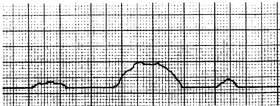
Figure 8.7: Response of the coagulating beam confocal reflectometer when small white dots on a black background target were passed slowly through the beam. The target was at the intended retinal plane.
