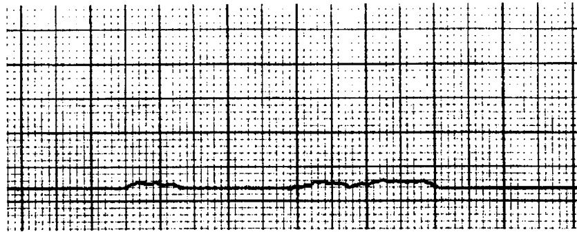
Figure 8.8: Response of the coagulating beam confocal reflectometer when small white dots on a black background target were passed slowly through the beam. The target was 10 mm further away than the intended retinal plane.
