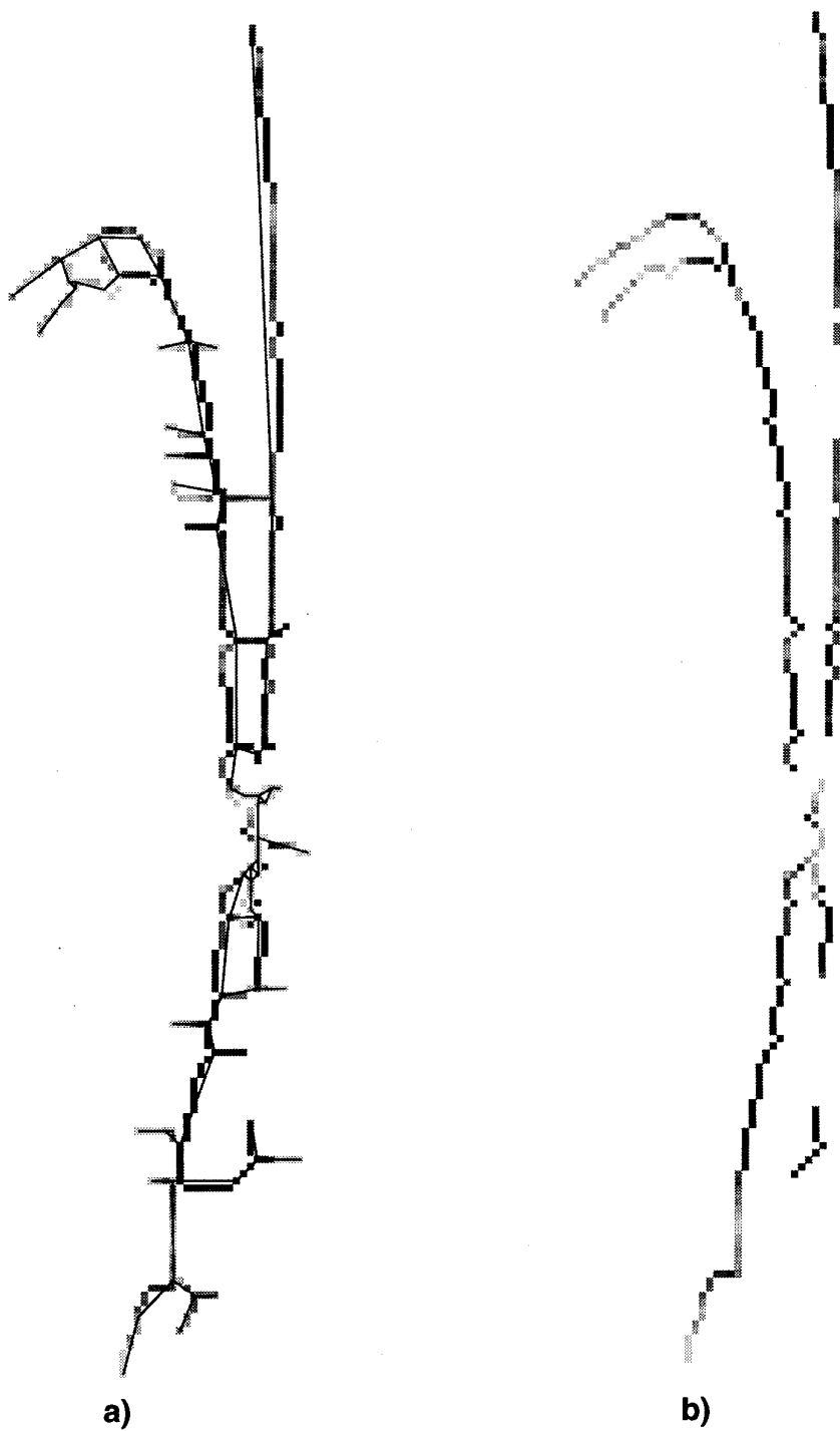
Figure 3.20: The advanced procedure for trimming a thinned ionogram trace. a) Piecewise-linear approximation to the trace structure. b) Final result.
