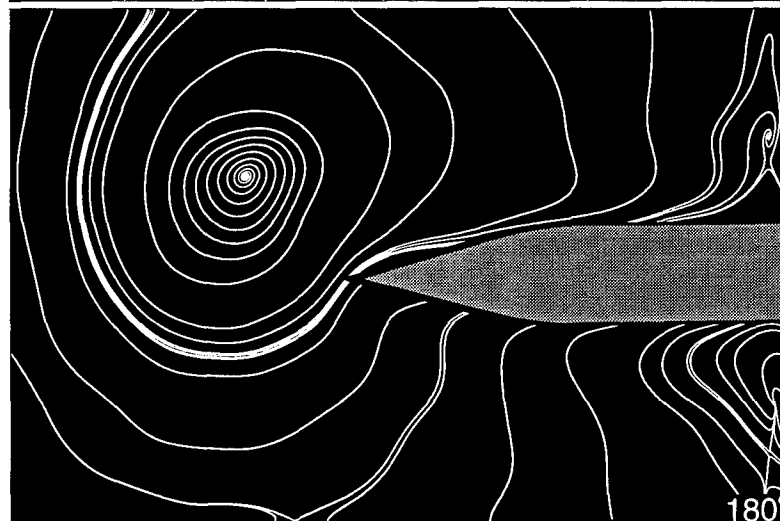
Figure 6.10: Instantaneous streamline patterns in a moving reference frame showing the interaction of an incident clockwise vortex with a stationary and oscillating leading-edge. Re = 6,250 .
