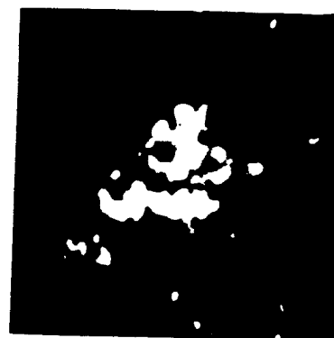
f) Aggregate: (513X) 35.7 \mu\text{m} X 36.1 \mu\text{m} 1.12 g/cc
