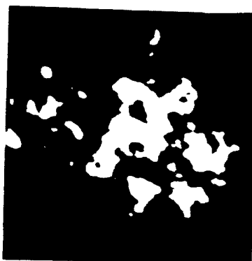
e) Aggregate: (513X) 54.2 \mu\text{m} X 52.4 \mu\text{m} 1.12 g/cc
