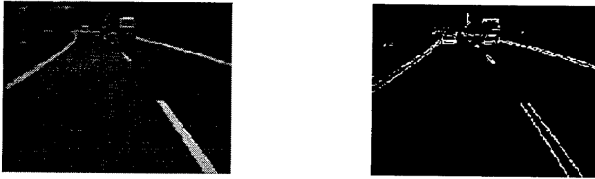
Figure 3: An example of an image with distant cars and its thresholded edge map.
